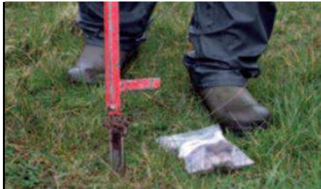
Soil testing auger and sample bags
