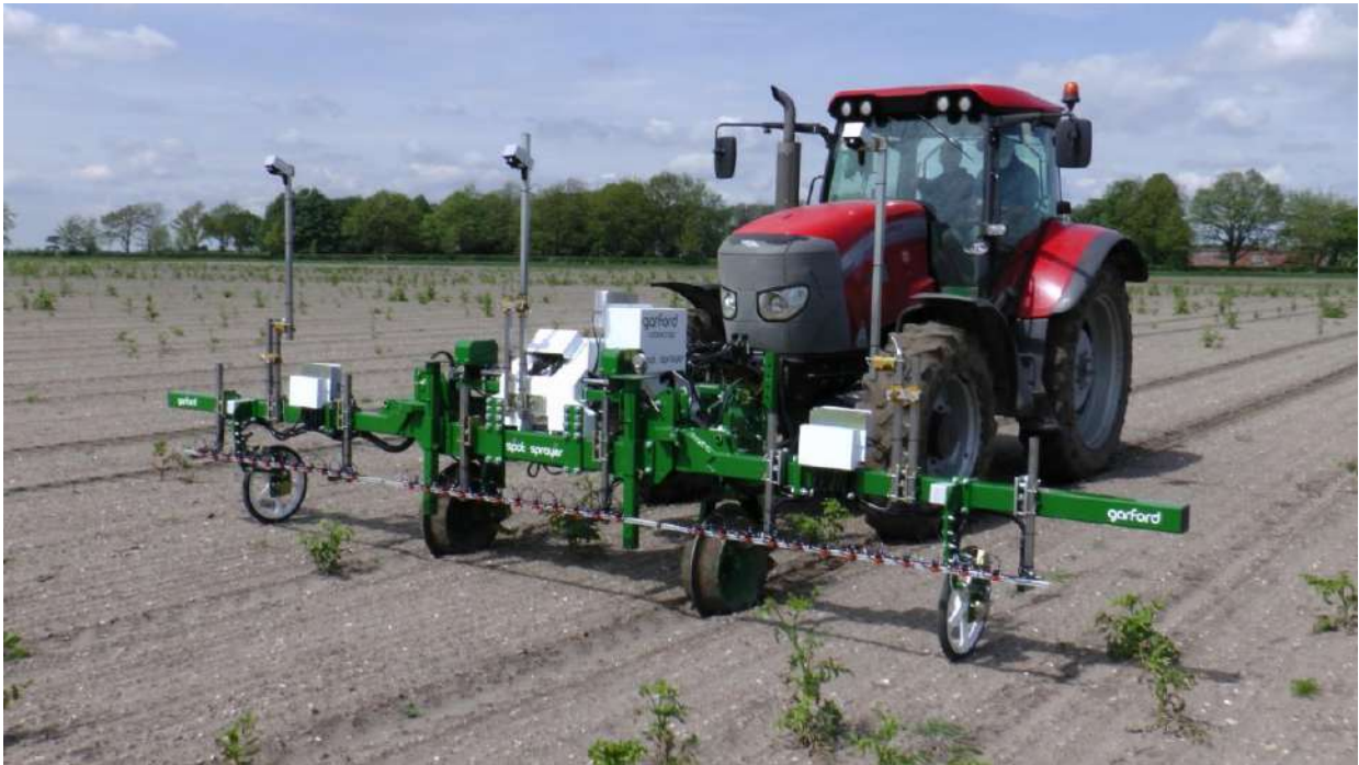
Robocrop spot sprayer tackling volunteer potato weeds in a young onion crop (image provided by Garford Farm Machinery Ltd)
