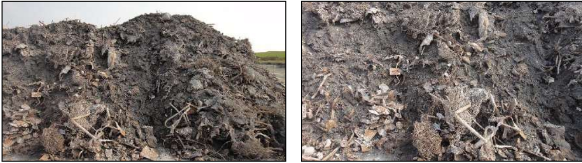
Plate 1. Raw IBA, no metal segregation, on Old Turkeyland maturation pad. April 2019 Rain falling on the maturation pad is routed to a run-off collection sump. This is a covered concrete tank buried in the ground adjacent to the north west corner of the pad. From here it is pumped to discharge to a sea outfall, under licence.
