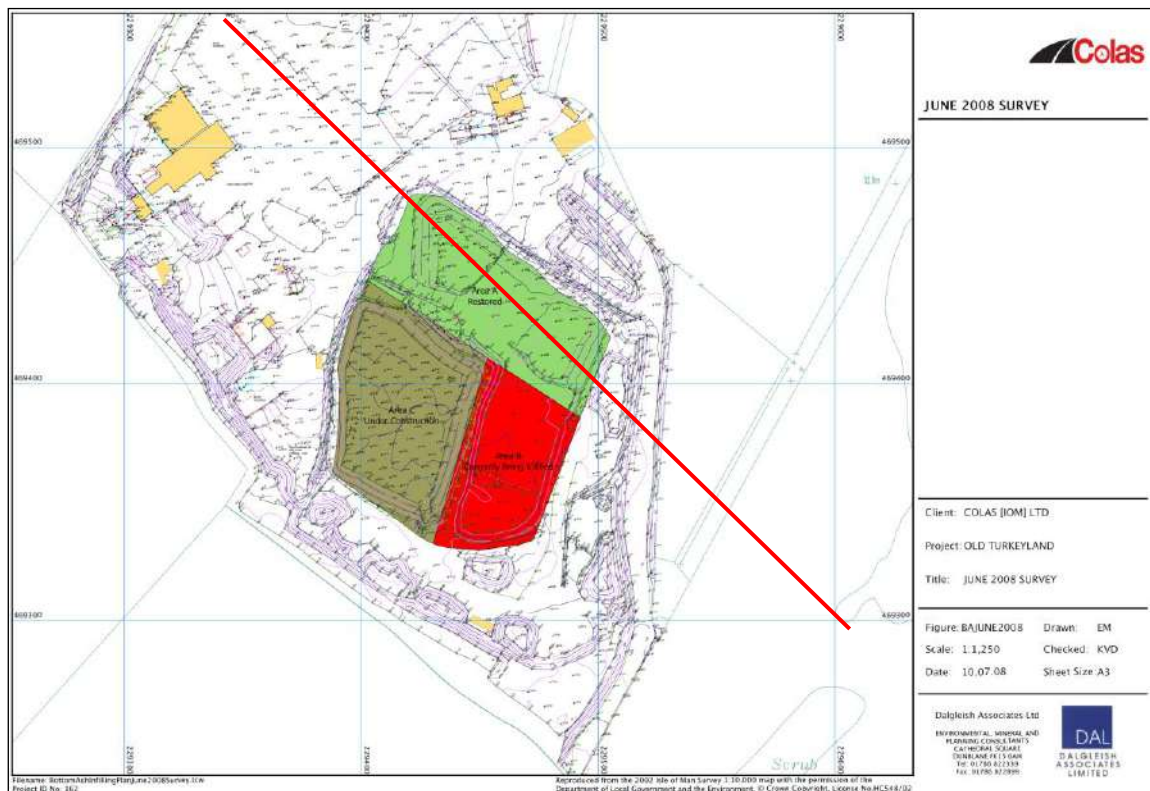
Figure 1-2 Layout of OTL landfill cells A to C, for IBA disposal, as at June 2008
