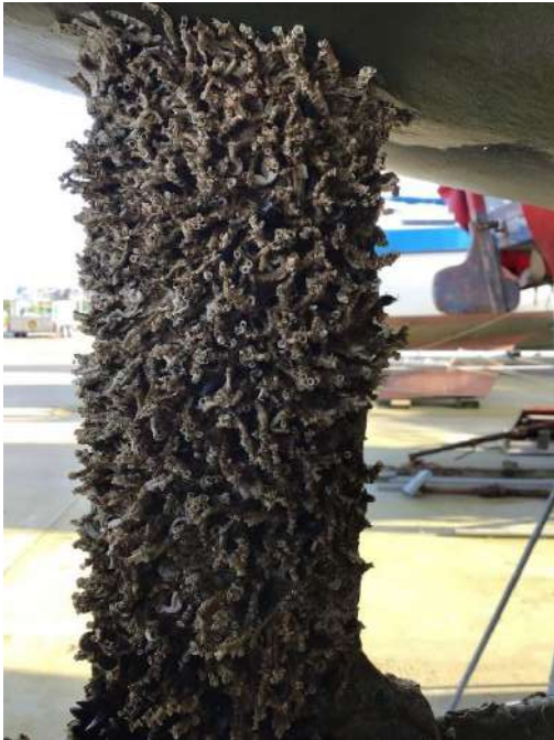
High profile (extended) form: mature colony growth with extended long tubes on metal parts of vessel steering/propulsion system. (Image: DEFA)
