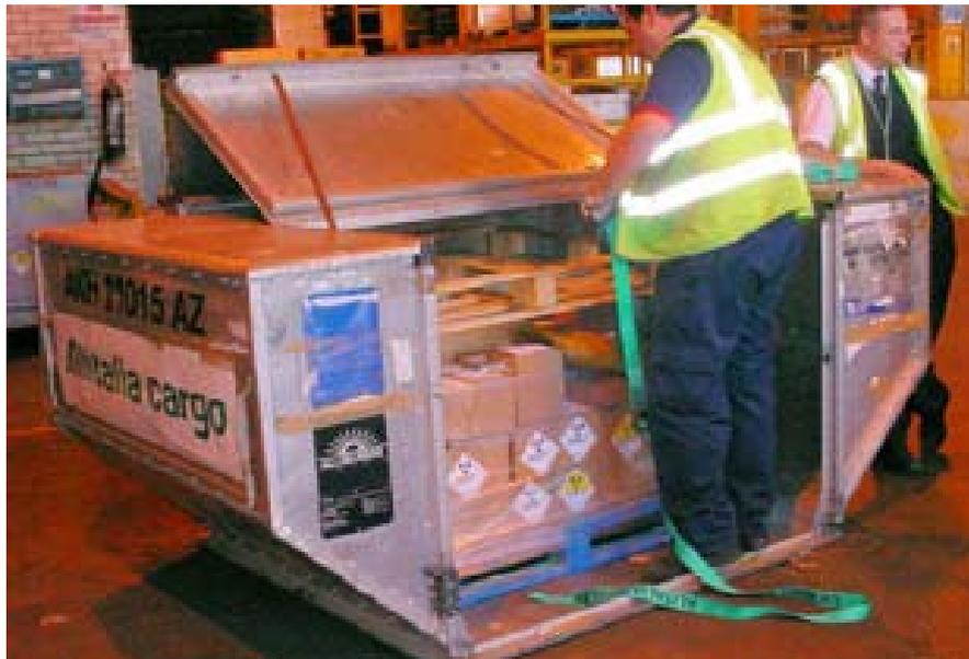
*Figure 6 – Unit Load Device*
