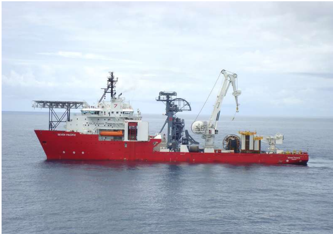
Vessel in Manx waters with cable and pipe laying kit on-board. Photo: Department for Enterprise.
