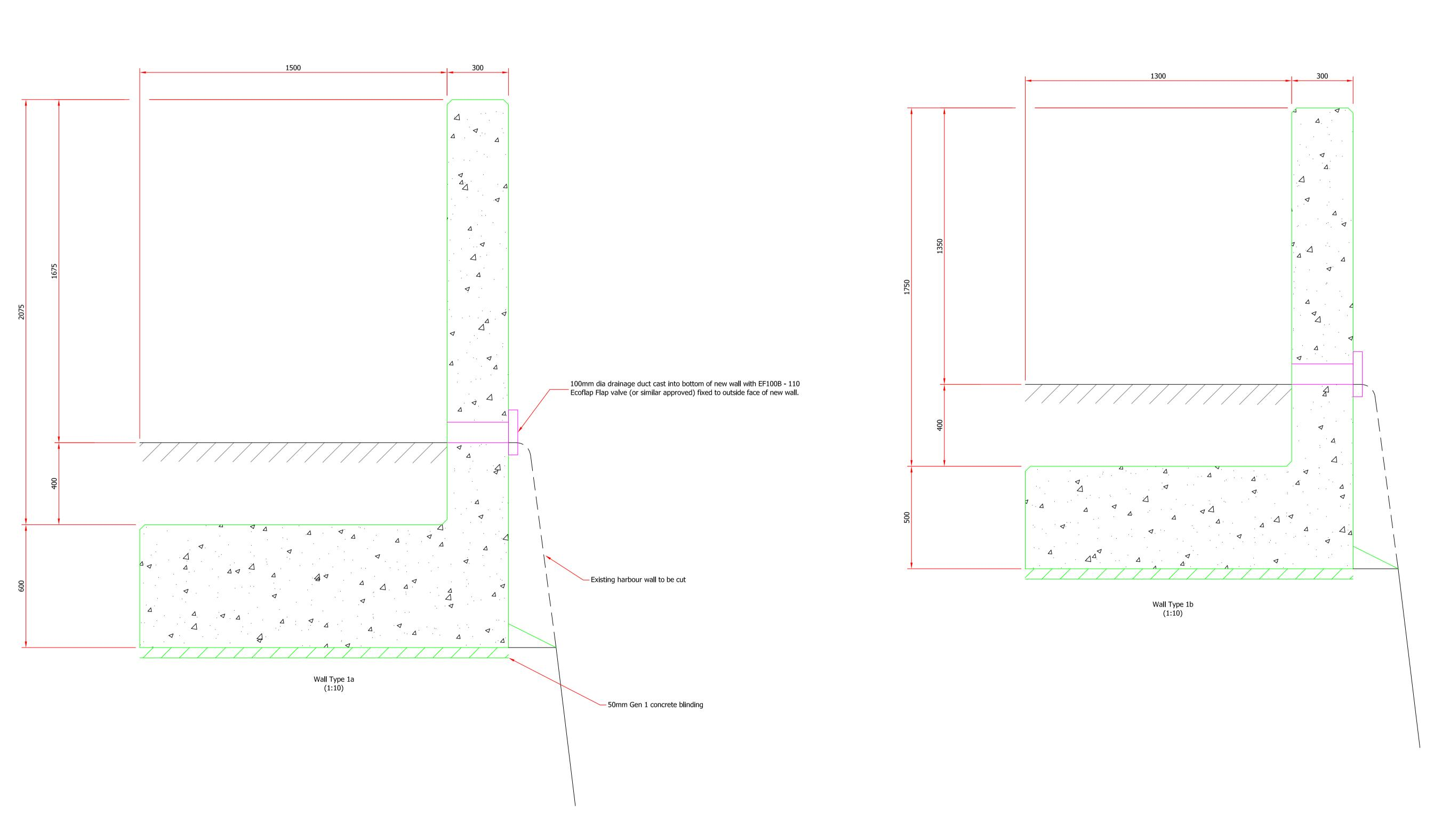
Boat Park wall stem height to be at 6.05m D02 unless stem would be less than 300mm from highway level. Minimum stem height to be 300mm.
