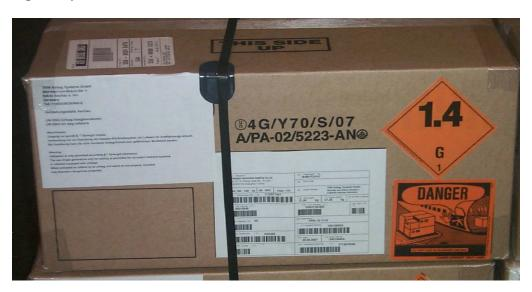
Figure 4 - Dangerous goods packing and labelling
