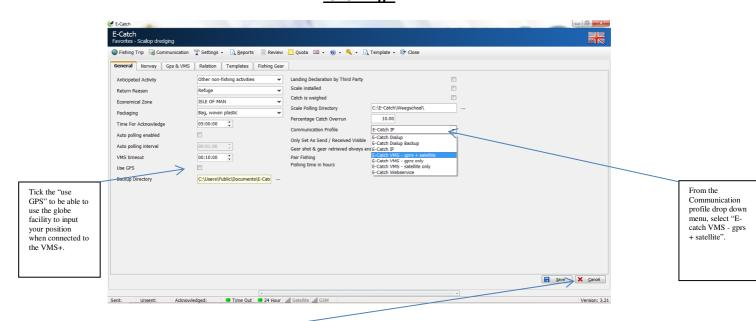
Finally save these settings and return to your fishing trip. You now have the ability to use the VMS+ to transmit your e-log providing that you have attached the cable from the VMS+ box to the USB connection on your laptop.
