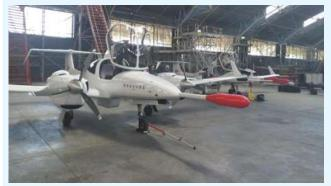
'Aerial work' is the conduct of specialised services such as survey, mapping or inspection. The 'M' registered DA42 aircraft pictured to the left are based in Africa to conduct aerial survey in support of mining operations.
