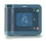
An automated external defibrillator (AED) is an emergency life-saving device for use in cardiac arrest. It is a portable appliance that analyses the heart rhythm and administers an electrical shock to the heart if needed which re-establishes a regular heart rhythm.
