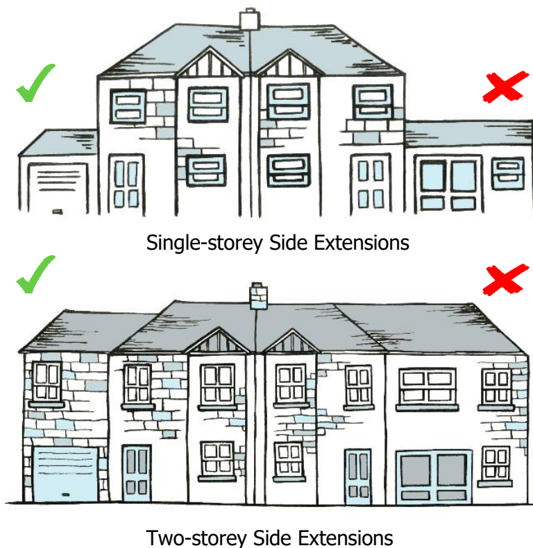
Figure 4.K: Side Extensions should Respect the Height and Width of the Main Dwelling
