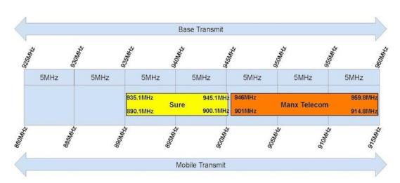
Figure 3: current spectrum assignments in the 900 MHz band
