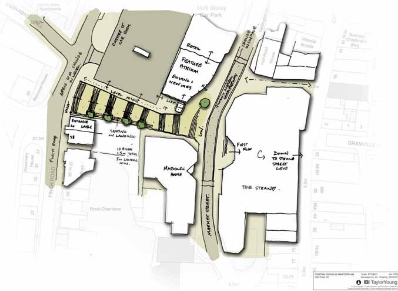
Figure 4 Indicative Sketch Scheme for Well Road Hill, looking at how better access can be achieved.
