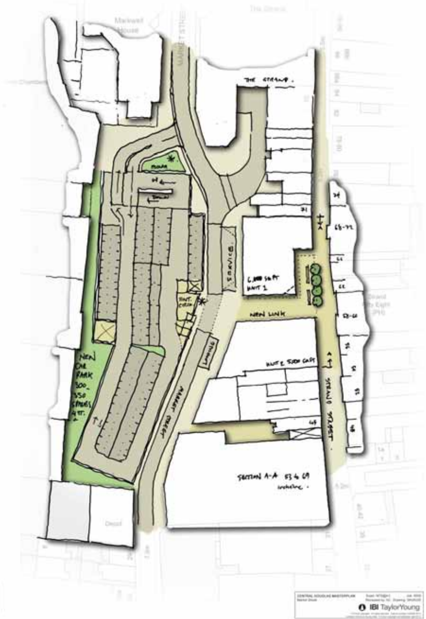
Figure 5 Indicative sketch scheme for Strand Street unit enlargement through the removal of existing units, and the opening up of the Market Street site.
