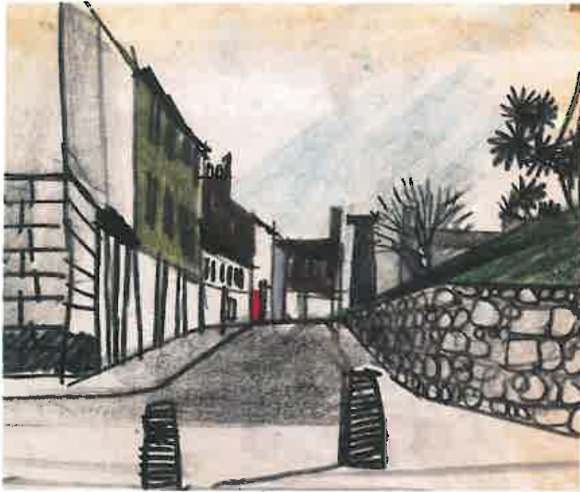
Glacis retaining wall made horizontal so that grass flows into Parade level at top of Castle Street which remains open to cars.
