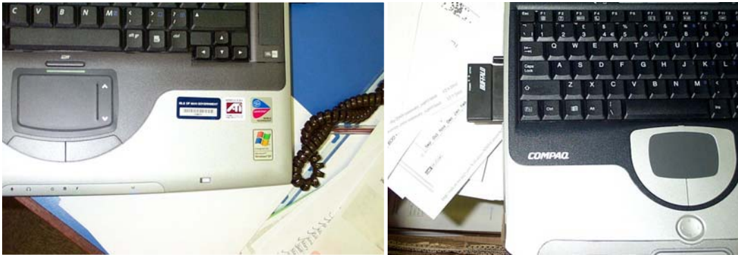
Picture 2 Laptop computers configured for wireless LAN with Centrino Mobile Technology (left) and a Buffalo card in the PCMCIA port (right)
